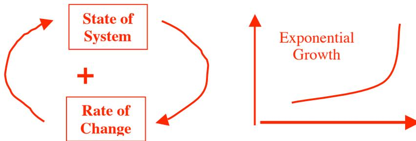
Figure Seven: Positive Feedback Loop Producing Exponential Growth Curve
